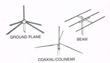
GROUND PLANE antenna is the most commonly used antenna for base stations. It is fairly effective, omni-directional, lightweight, easy to mount, and economical. It is designed for medium-long range communications.
