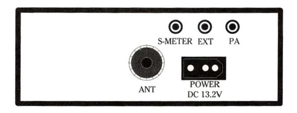
Connect the power cord supplied with the radio to a source of 12 Volts DC. Connect the red wire to the (+) side and the black wire to the (-) side.
