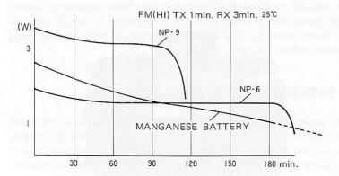
The voltage/power versus time characteristics is shown in the above illustration. SSB operation normally extends battery life 3 to 4 times longer than FM. Also, use of low power reduces battery consumption resulting in longer operating life.
