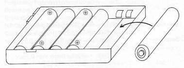
\* Be sure to insert batteries with correct polarity.
