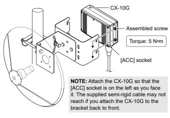
6 Loosen the nuts to adjust the angle of the AH-109PB. After adjusting, tighten the nuts again.
