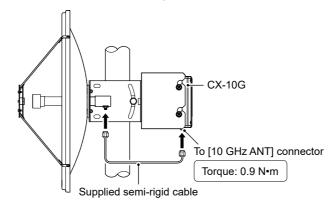
**TIP:** After connecting, covering the connectors with a rubber vulcanizing tape prevents water from seeping into the connection.
