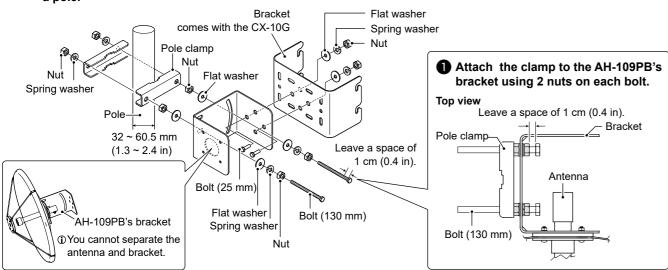
4 Attach the CX-10G to the bracket, and then tighten the assembled screws.
