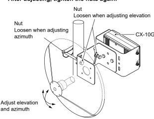
**NOTE:** When adjusting azimuth, be careful not to loosen the nuts too much causing the antenna to fall.
