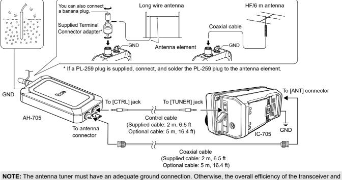
antenna tuner installation will be reduced. Interference, RF feedback, and electrical shocks from other equipment could also occur.
